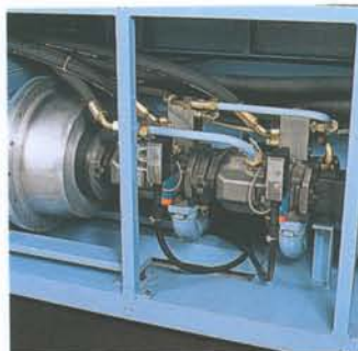
Due pompe a portata variabile Variable displacement servo-pumps Servopompes Servo-bombas
